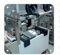
The PRS unpacking station is also a basic feature of the SLM®500HL. This useful component of the system is optimally suited for batch production, and serves for removing the manufactured components properly from the construction cylinder under an inert gas atmosphere.
