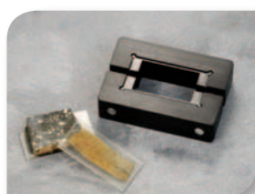
Petrographic glass slide hand-held holder for 27 x 46mm glass slides
